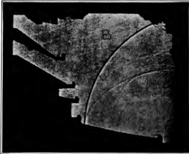
FIG. 71. Position of a sound wave in a theater \frac{1}{10} second after its production on the stage.
